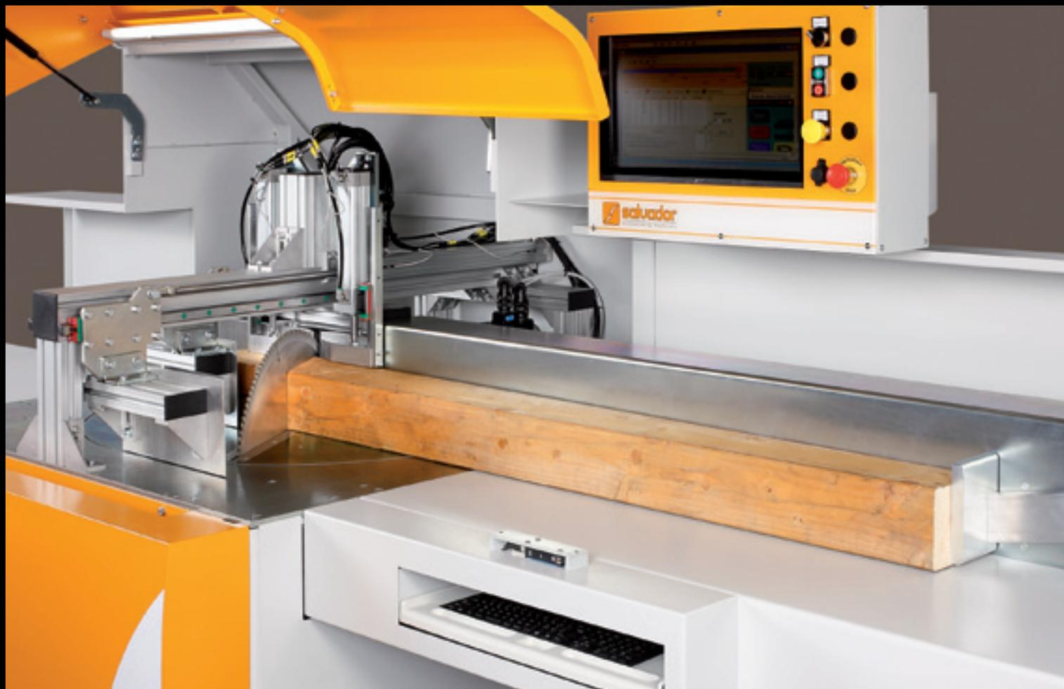
**Fast and precise:** the rotating table is fixed on an innovative high precision mechanical construction system that guarantees exact angles and it is managed directly by an electronic motor of high technology and power also during braking. Only thanks to the combination of these two innovative and highly technological solutions, Superangle 600 obtains at the same time the maximum precision with the maximum speed of movement.
