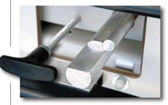
The heavy duty mid fence has, just as the bottom beam, a handy end stop. This prevents the slipping of the panel when cutting horizontally.
