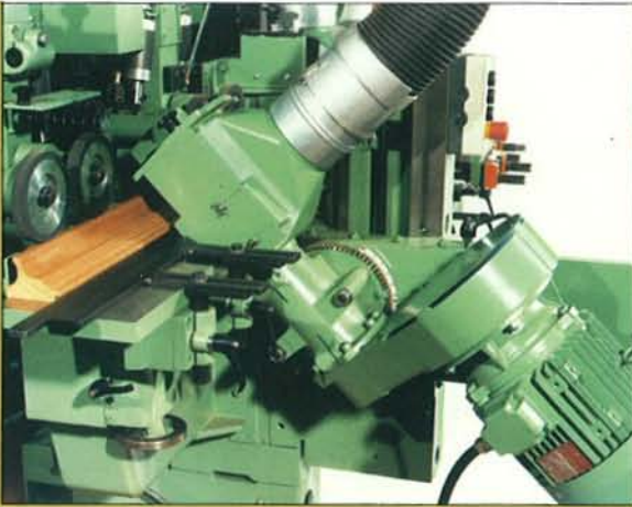
△ The optional 3 and 4 position universal heads allow complete moulding flexibility (can be fitted at a later date if required).
