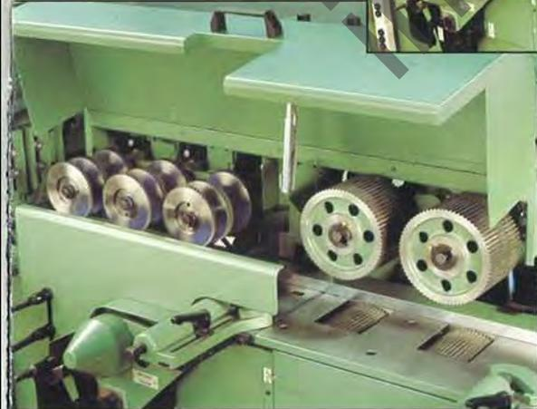
△ Effortless feeding of thin and difficult material up to 120m/min, guaranteed with top and bottom feed rolls throughout the machine.
