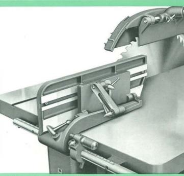
The robust canting fence has quick hand adjustment across the table with screw adjustment for fine setting. It pivots on centres, the one nearest the saw being eccentric to allow the fence to be adjusted towards or away from the saw. Fence swings clear of the table for cross cutting.
