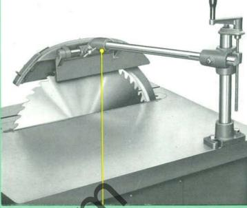
Saw guard has screw use and fall and gives protection to both edges of saw. Cover turns over for access to saw.
