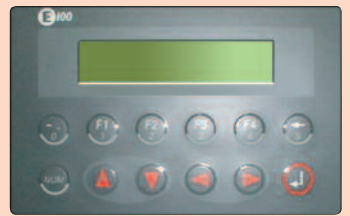
HMI Control Unit
