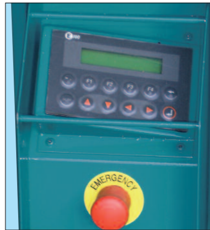
HMI Control Unit
