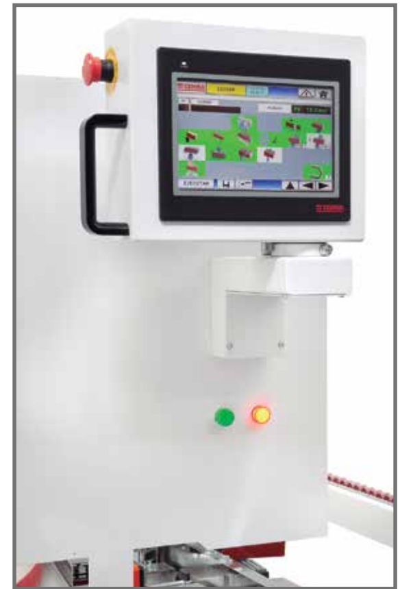
The edgebander is managed with a big Color Touch Screen
